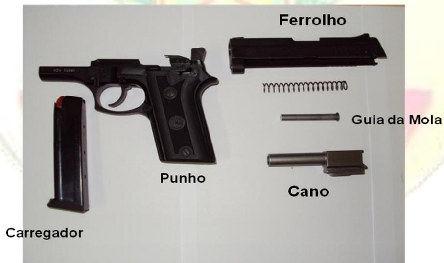
**VISTA DESMONTADA****FERROLHO****GUIA DA MOLA****MOLA RECUPERADORA****CANO****ARMAÇÃO****CARREGADOR**
